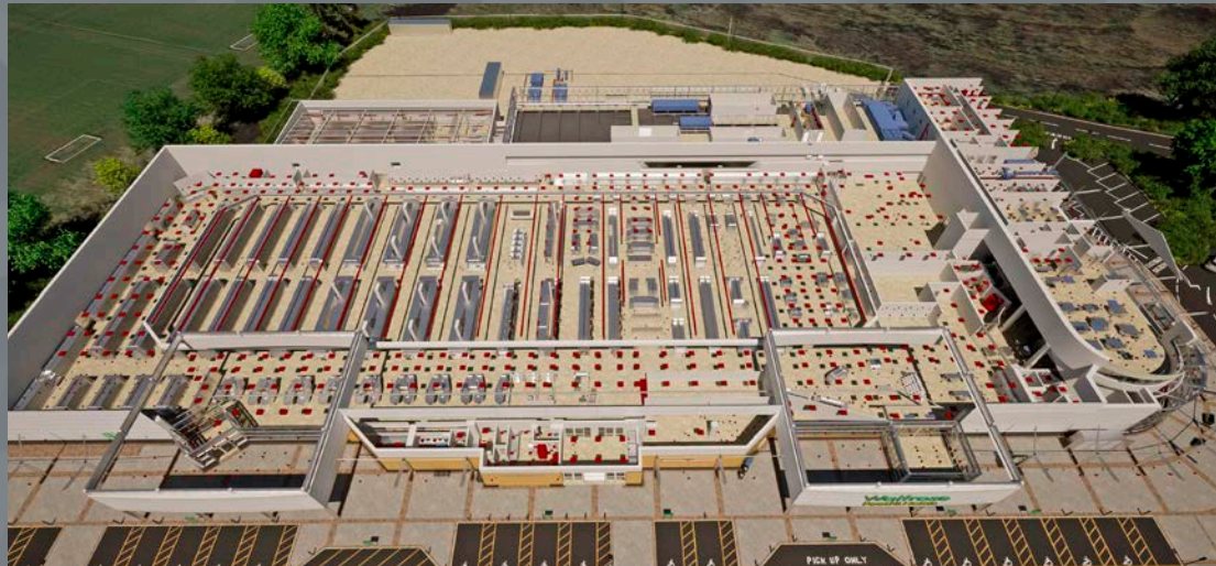
Internals modelled to LOD300 including shop layout and building services
